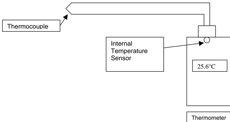
Inside the thermometer the CJC sensor is located as close as possible to where the metal of the thermocouple changes to copper, Note that thermocouples are supplied with special plugs (colour coded) made of the same metals of the thermocouple itself. If it is necessary to extend a thermocouple then it can only be extended with the same metal. The whole effect of a thermocouple is due to connecting different metals together, so great care must be taken to avoid large errors.
