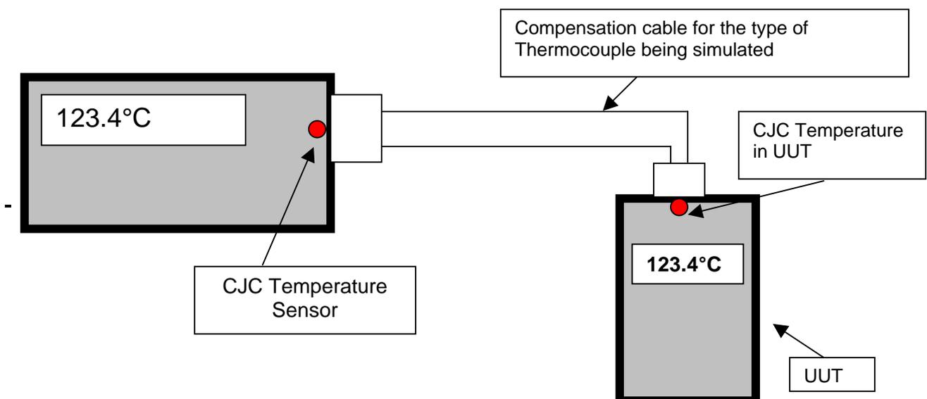
This method still requires characterised compensation cable for each type of thermocouple to be simulated. Additional uncertainties are introduced from the errors in using compensation cable between the UUT and the CJC in the calibrator. Also as the calibrator will have self-heating the error is greater due to the thermal gradient across the cable and plugs producing thermal emf.
