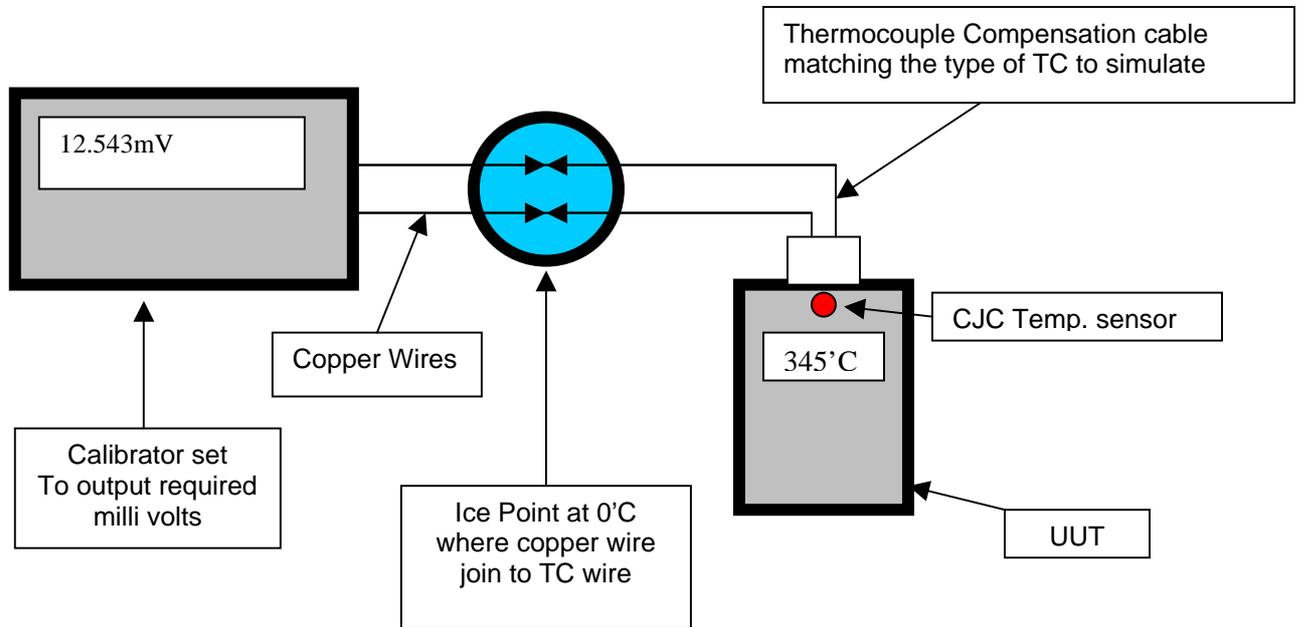
This method is accurate, but requires an ice point reference and also characterised Thermocouple compensation wire is needed for each type of TC to simulate.
